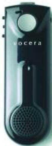
A wearable 2 oz communications badge is part of a communications system from Vocera ( www.vocera.com ) that allows hospital staff to speak instantly to the resource they need.
